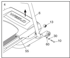
5. Hold the Console Base (1) near the Right Handrail (6). **Touch the Right Handrail to discharge any static.**
